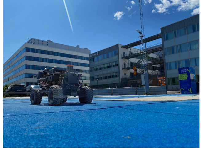
Fig. 1. A snapshot of the 1/10th-scale SVEA platform driving in the presented 5G-based C-V2X testbed in the Kista Innovation Park. More details about the SVEA platform at https://svea.eecs.kth.se
