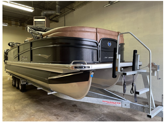
Fig. 2. Test boat: Premier Intrigue of 2022 model year. Specifications are with overall length of 8.36 [m], beam length of 3.1 [m], and dry weight of 3,500 [lb].
