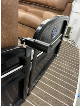
Fig. 4. The camera installed at the bow of the pontoon. Specifications: 2880x1860 of resolution, 6.9 [FPS], 8 [mm] of focal length, 58.4 [deg] of FOV.
