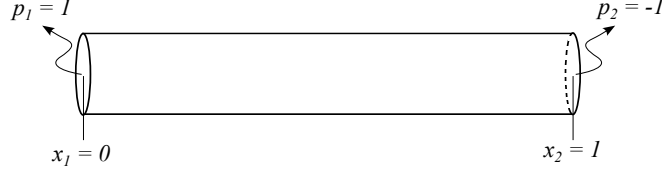
Figure 3: Schematic diagram of a uniform duct with boundary conditions.
