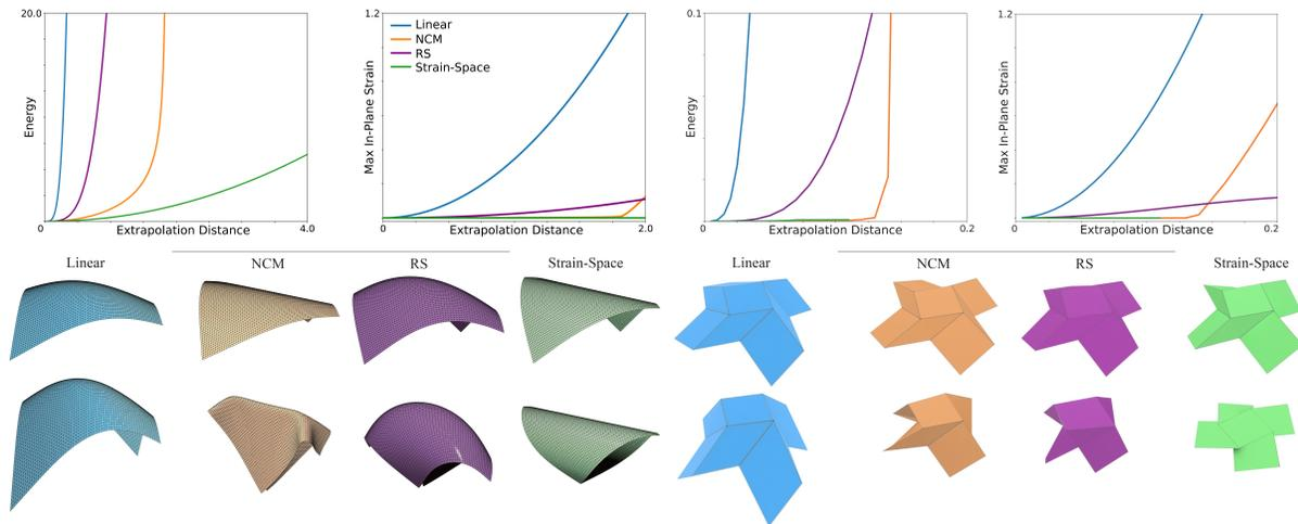
**Figure 3: Comparing internal energy and maximum in-plane strain along the first non-rigid mode computed using linear eigenmodes, nonlinear compliant modes (NCM), rotation-strain modes (RSM), and our strain-space modes.**
