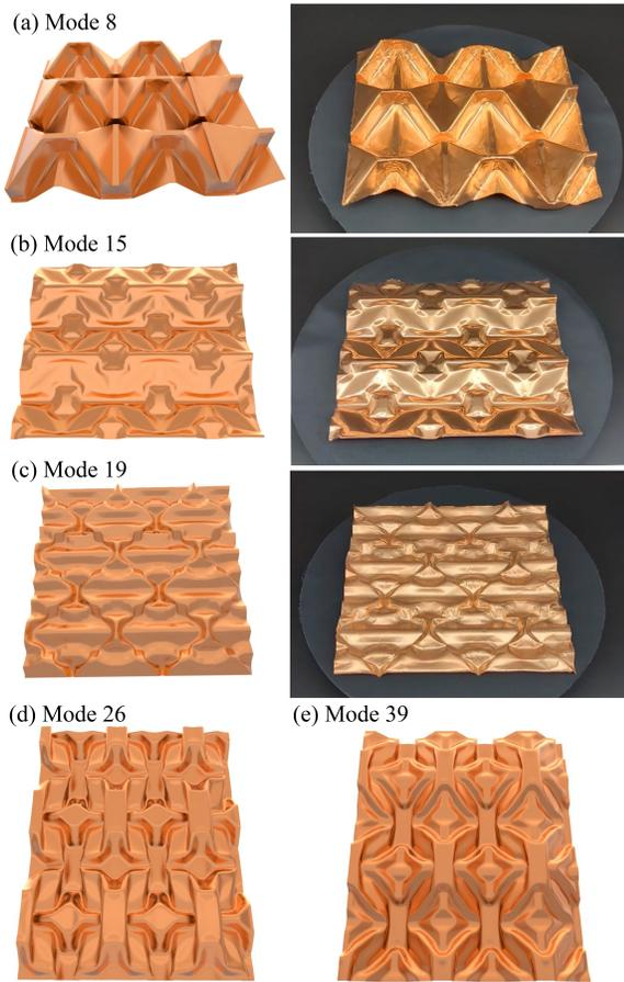
**Figure 2: Periodic folding patterns obtained using Modal Folding (a-e) with reflection boundary conditions and their corresponding physical prototypes (right) manufactured using copper sheets and 3D-printed press dies.**
