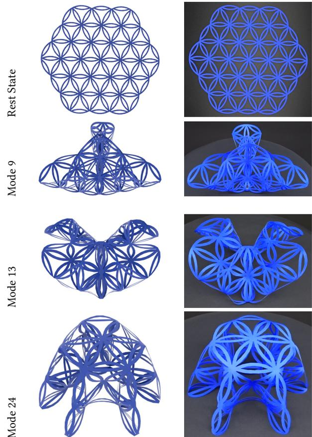
Figure 6: Folding patterns for a thin sheet cut into the pattern of a life flower.
