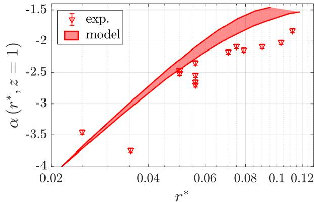
Figure 17: Here  $\alpha$  versus  $r^*$  for  $Ja = 0.5$  and  $Ha = 3.8 \times 10^4$ . Here  $r^*$  is the distance in the  $(x, y)$  plane between a given measurement location and the nearest injection electrode.
