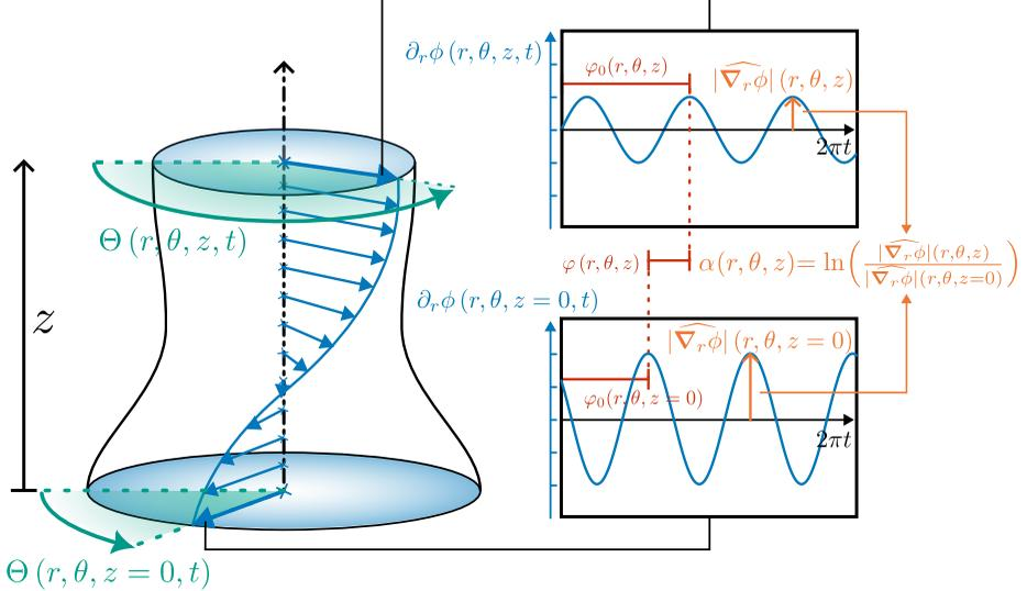
Figure 3: Illustration of the different diagnosis quantities for the oscillating flow: the local phase shift  $\varphi(r, \theta, z) = \varphi_0(r, \theta, z) - \varphi_0(r, \theta, z=0)$ ; the local attenuation coefficient  $\alpha(r, \theta, z) = \ln \left( \frac{|\nabla_r \phi(r, \theta, z)|}{|\nabla_r \phi(r, \theta, z=0)|} \right)$ ; the horizontal polar angle  $\Theta(r, \theta, z, t)$  of the horizontal electric potential gradient  $\nabla \phi$ .
