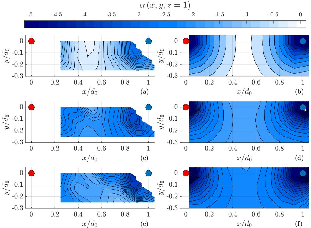
Figure 15: Snapshot contours of  $\alpha$  at the top wall ( $z = 1$ ) for  $Ja = 0.1$  (a, b),  $Ja = 0.5$  (c, d) and  $Ja = 1$  (e, f). Here  $Ha = 3.8 \times 10^4$  for all cases. For each value of  $Ja$ , contours of  $\Theta$  are plotted from experimental data (a, c, e) and from the propagative low- $Re$  model (b, d, f). The coloured circles show the location of two electrodes in phase opposition out of the four injection electrodes.
