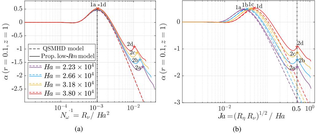
Figure 4: Attenuation coefficient  $\alpha$  against  $N_{\omega}^{-1}$  (a) and  $Ja$  (b) for  $Ha = \{1.9 \times 10^4, 2.66 \times 10^4, 3.18 \times 10^4, 3.8 \times 10^4\}$ : solid lines (—), propagative low- $Rm$  model; dashed lines (---), QSMHD model. Calculations are performed at  $r = 0.1$ . The attenuation coefficient  $\alpha$  is calculated at  $z = 1$ .
