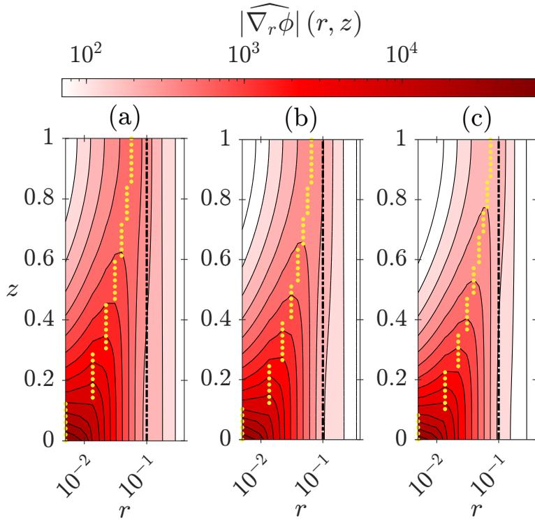
Figure 8: Contours of  $|\widehat{\nabla_r \phi}|$  from the QSMHD model at  $Ha = 3.8 \times 10^4$  and for  $N_\omega^{-1} = \{(a) 0.75; (b) 1; (c) 1.25\} \times 10^{-3}$ . The dotted line ( $\cdots$ ) shows the radial location  $r_m(z)$  of the maximal velocity.
