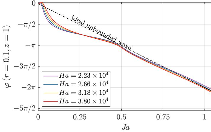
Figure 10: Phase shift  $\varphi$  from the propagative low- $Rn$  model against  $Ja$  at  $r = 0.1$  for  $Ha = \{1.9 \times 10^4, 2.66 \times 10^4, 3.18 \times 10^4, 3.8 \times 10^4\}$ . The dash-dotted line (---)  $\varphi$  is for an ideal unbounded wave.
