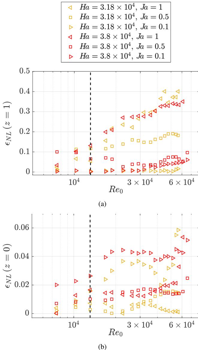
Figure 19: Normalised  $\langle |\widehat{\nabla_x \phi}| \rangle$  against  $Re_0$  at the top wall (a) and the bottom wall (b) for  $Ha = \{3.18 \times 10^4, 3.8 \times 10^4\}$  and  $Ja = \{0.1, 0.5, 1\}$ . For each case of the set  $\{Ha, Ja\}$ ,  $\langle |\widehat{\nabla_x \phi}| \rangle$  is normalised by its value at the lowest experimental  $Re_0$ .
