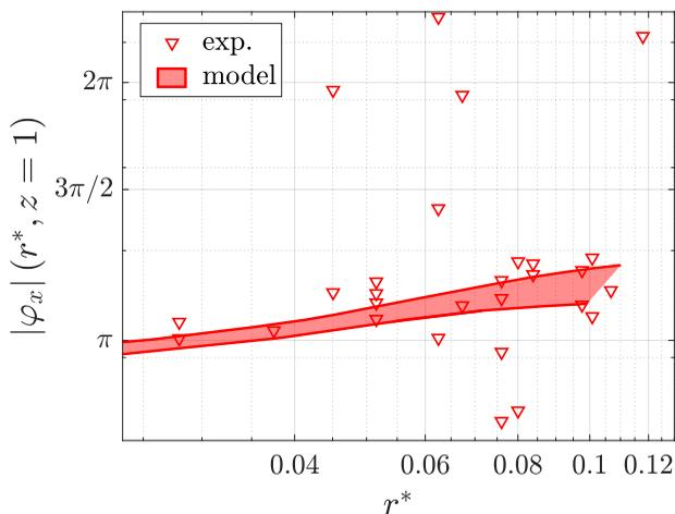
Figure 18: Here  $\varphi_x$  against  $r^*$  for  $Ja = 0.5$  and  $Ha = 3.8 \times 10^4$ . Here  $r^*$  is the distance in the  $(x, y)$  plane between a given measurement location and the nearest injection electrode.
