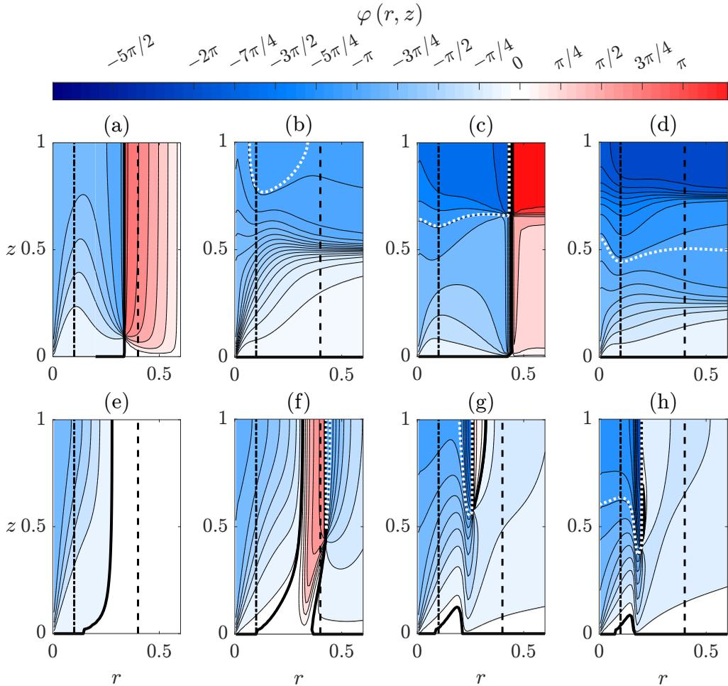
Figure 7: Contours of  $\varphi$  at  $Ha = 3.8 \times 10^4$  and for  $Ja = \{(a, e) 0.25; (b, f) 0.5; (c, g) 0.75; (d, h) 1\}$ : (a–d) propagative low- $Rn$  model; (e–h) QSMHD model. The solid line (—) marks the  $\varphi = 0$  iso-value and the dotted line (····) the  $\varphi = -\pi$  iso-value.
