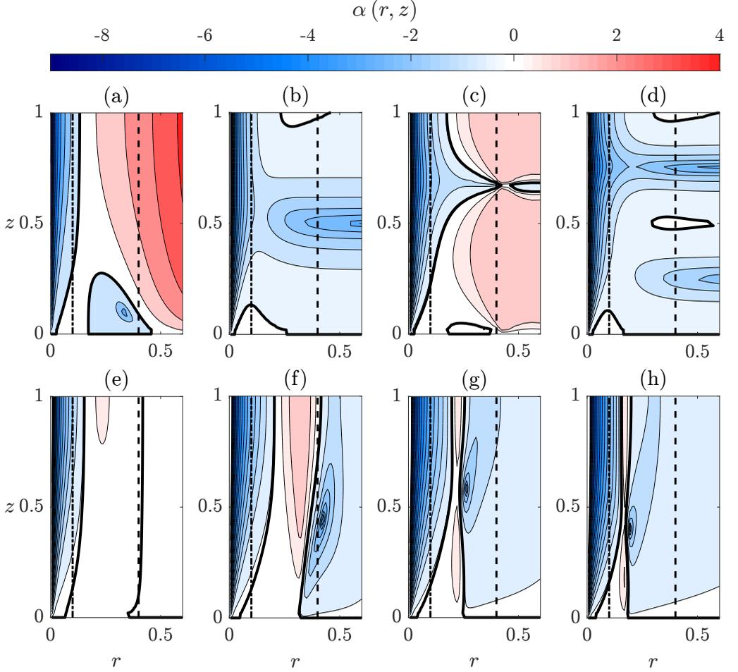
Figure 6: Contours of  $\alpha(r, z)$  at  $Ha = 3.8 \times 10^4$  and for  $Ja = \{(a, e) 0.25; (b, f) 0.5; (c, g) 0.75; (d, h) 1\}$ ; (a–d) propagative low- $Rn$  model; (e–h) QSMHD model. The vertical dash-dotted line (---), indicates the radial position  $r = 0.1$  where values of  $\alpha$  are taken for figure 4. The solid line (—) is the locus of  $\alpha(r, z) = 0$ .
