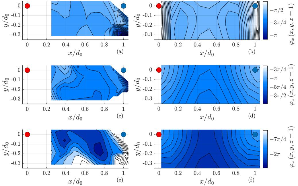
Figure 16: Snapshot contours of  $\varphi_x$  at the top wall ( $z = 1$ ) for  $Ja = 0.1$  (a, b),  $Ja = 0.5$  (c, d) and  $Ja = 1$  (e, f). Here  $Ha = 3.8 \times 10^4$  for all cases. For each value of  $Ja$ , the contours of  $\Theta$  are plotted from experimental data (a, c, e) and from the propagative low- $Rm$  model (b, d, f). The coloured circles show the location of two electrodes in phase opposition out of the four injection electrodes.
