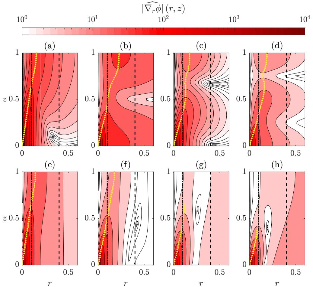
Figure 5: Contours of  $|\widehat{\nabla_r \phi}|$  at  $Ha = 3.8 \times 10^4$  and for  $Ja = \{(a, e) 0.25; (b, f) 0.5; (c, g) 0.75; (d, h) 1\}$ : (a–d) propagative low- $Rn$  model; (e–h) QSMHD model. The vertical dash-dotted line (---) is located at  $r = 0.1$  and the vertical dashed line (---) at  $r = 0.4$ . The dotted line (.....) shows the radial location  $r_m(z)$  of the maximal velocity.
