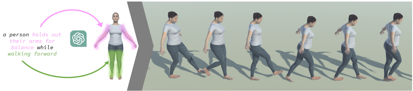
Figure 1: LGTM decomposes input text description at the part level using LLMs and generates output motion from local to global with both part description and full-body descriptions.
