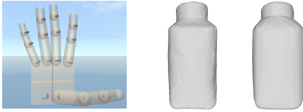
Figure 3: Our physical hand model (Left), object mesh reconstructed from kinematic tracking (Middle), and convex object collision mesh (Right).
