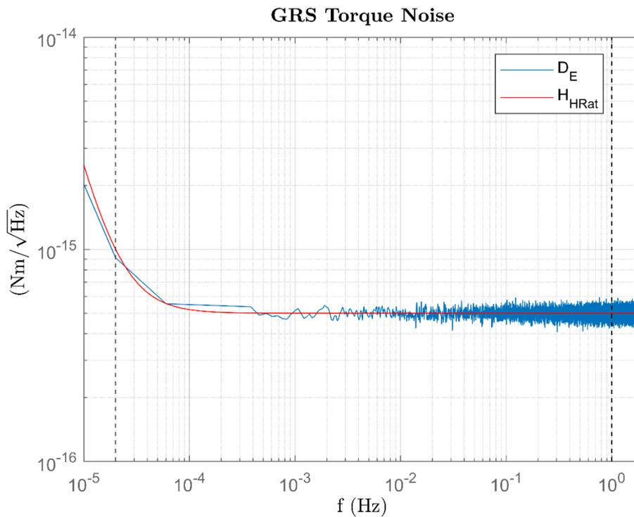
Figure 2 – GRS Torque Noise. Blue: simulated, red: shape filter.
