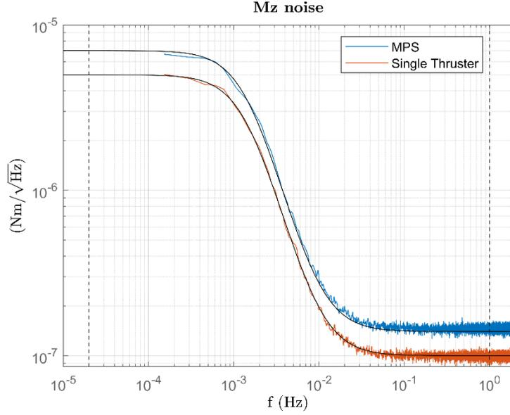
Figure 4 – MPS torque noises. Red: single thruster. Blue: MPS system
