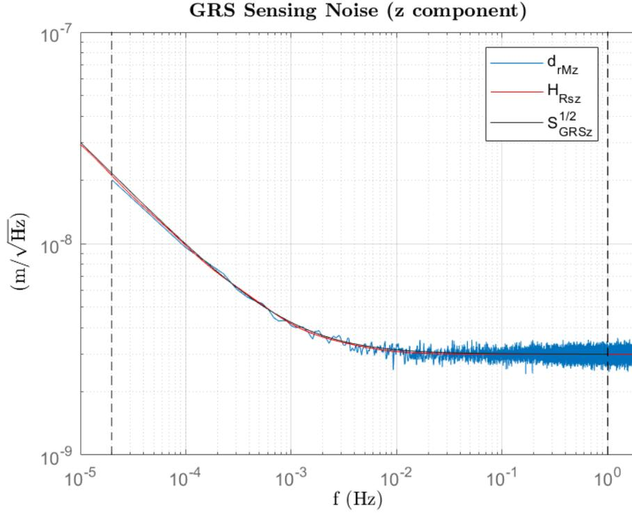
Figure 7 - GRS sensing noise (vertical position). Blue: simulated, red: shape filter
