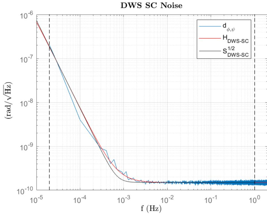
Figure 10 – DWS SC sensing noise (azimuth-elevation). Blue: simulated, red: shape filter
