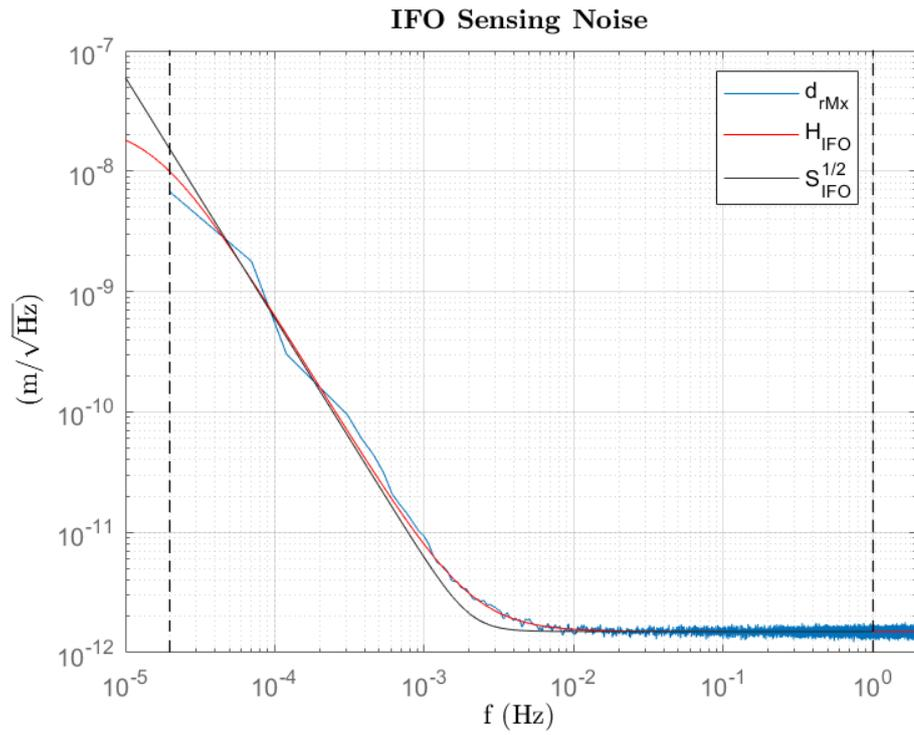
Figure 5 – Interferometer sensing noise. Blue: simulated, red: shape filter
