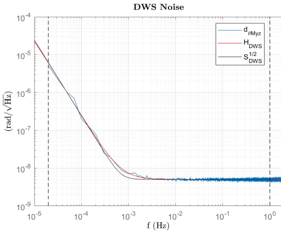
Figure 9 – DWS sensing noise (test-mass pitch/yaw). Blue: simulated, red: shape filter
