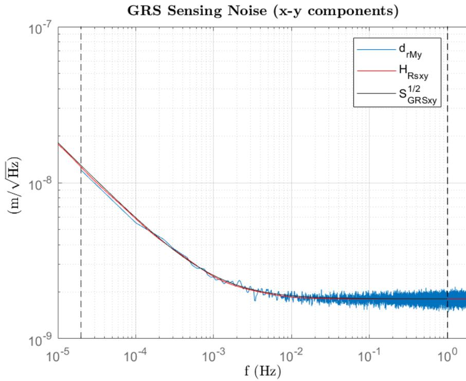
Figure 6 – GRS Sensing Noise (longitudinal and lateral position). Blue: simulated, red: shape filter
