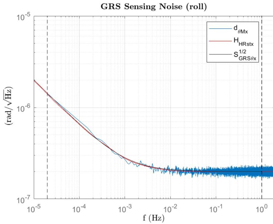
Figure 8 – GRS sensing noise (test-mass roll). Blue: simulated, red: shape filter
