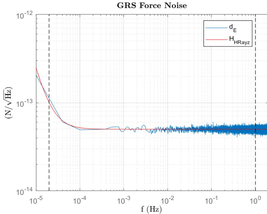
Figure 1 – GRS Force Noise (y-z component). Blue: simulated, red: shape filter.
