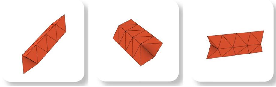
**Fig. 14** Various views of the 3-cushion consisting of three octahedra and 8 tetrahedra
