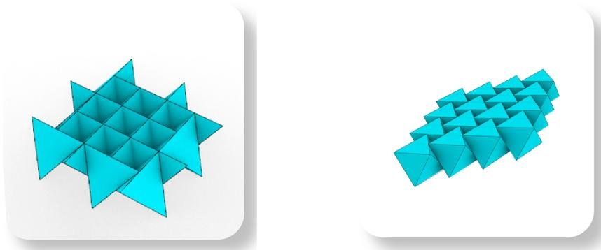
**Fig. 6** Tetrahedra- and octahedra-interlocking assemblies, see (Dyskin et al., 2003a)
