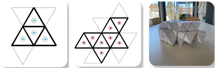
**Fig. 3** (Left, middle) Folding plans for the tetrahedron and octahedron with  $+$ ,  $-$  signs according to the poling; (right) a block constructed by assembling tetrahedra and octahedra with inserted magnets
