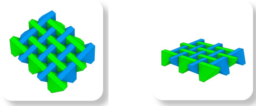
**Fig. 29** Various views of the assembly of the truncated tetrahedron also called flat Abeille vault in literature
