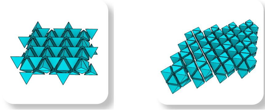
**Fig. 8** Exploded view of tetrahedra and octahedra TI assemblies inside the tetrahedral-octahedral honeycomb
