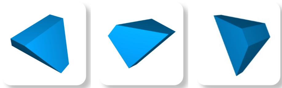
**Fig. 28** Truncating two opposite edges of a tetrahedron leads to the Abeille block, see ([Gallon, 1735](#))
