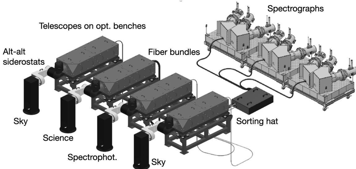
**Figure 2.** The LVM-I instrument and its major subsystems.
