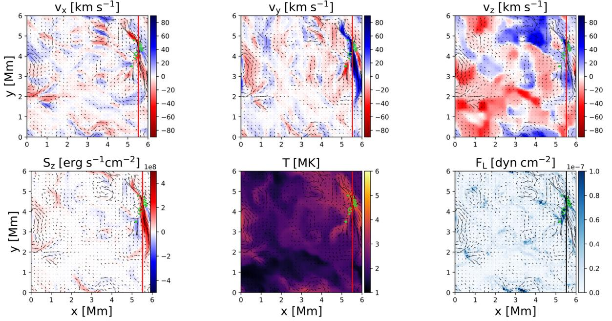
**Figure 8.** Cuts perpendicular to the loop axis at the location of slit 5 for event (a). Top row: x, y and z component of the velocity. Bottom row: Axial Poynting flux, temperature, and horizontally directed Lorentz force. The arrows illustrate the velocity field. The solid red line indicates the position of the peak in line width for this event. The green contour outlines regions with a heating rate of  $\log_{10}(Q_{tot}) > -1$ .
