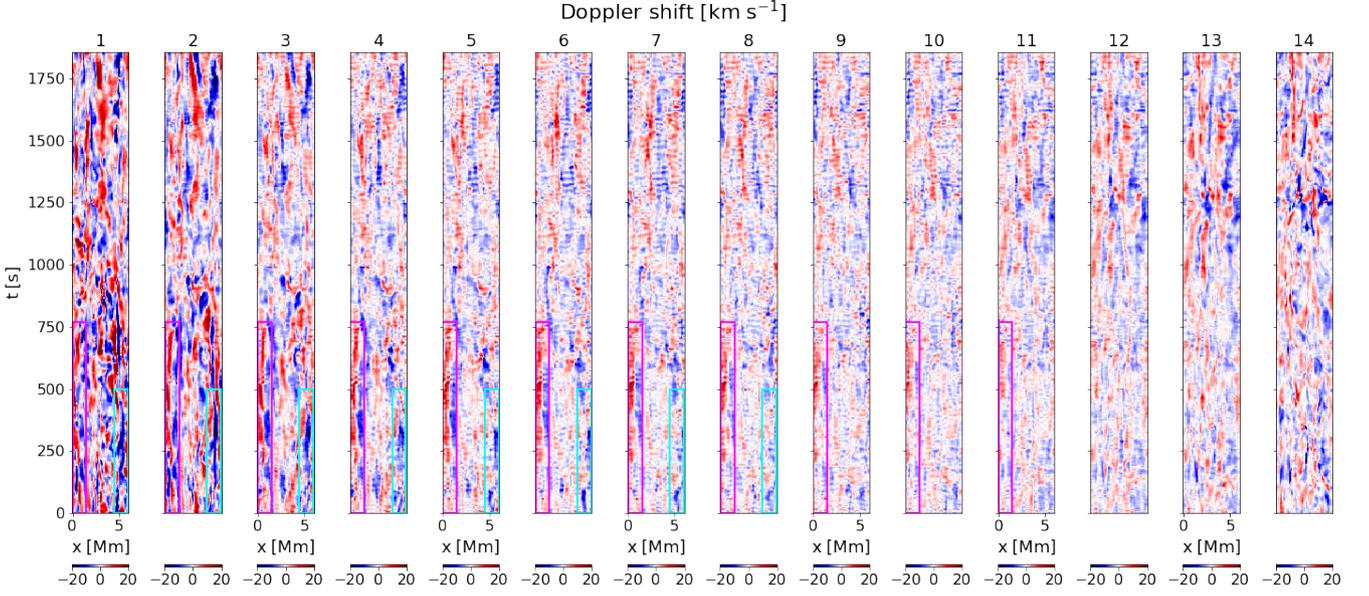
**Figure 3.** Synthetic "sit and stare" observation for 14 of the 35 MUSE slits. From left to right, the figure shows time-distance plots of the Doppler shift at each slit. The location of the slits is marked by the dashed black lines in Fig. 1. The pink and blue boxes mark the location of long-lived strong Doppler shifts.
