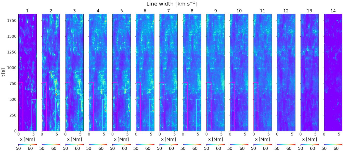
**Figure 4.** Synthetic "sit and stare" observation for 14 of the 35 MUSE slits. From left to right, the figure shows the time-distance plots of the line width at each slit. The location of the slits is marked by the dashed black lines in Fig. 1. The pink and blue boxes mark the location of long-lived strong Doppler shifts.
