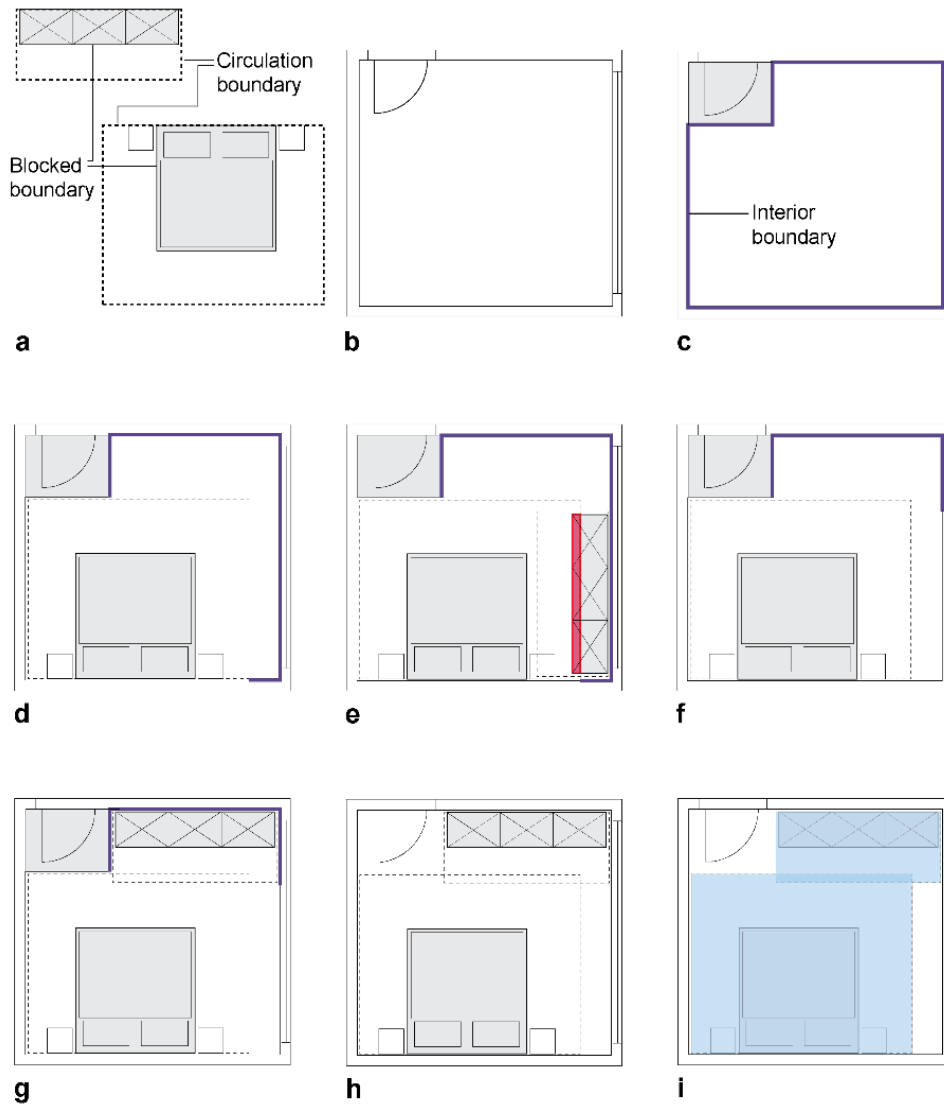
Supplemental Figure 6: Procedure of furniture placement inside a sample room. Furniture objects are defined with a circulation boundary that is allowed to intersect with other circulation boundaries and blocked boundary that is not allowed to intersect with any object (a). A bed and drawer are placed in the bedroom (b). The circulation area of the door is subtracted from the interior boundary to create the interior placement polygon (c). The first furniture item (the bed) is placed along the first edge of the interior placement polygon (d) after successful placement the circulation bounds are subtracted from the interior boundary. The second furniture item (the drawer) is placed along the next line segment of the interior boundary. The blocked boundary of the drawer intersects with the circulation boundary of the bed (e), which is an infeasible placement. The interior boundary is shortened by the circulation boundary of the drawer (f), and in a second try the drawer is placed on the next line of the interior boundary polygon (g). A successful placement is achieved (h) and the furniture area of the room can be calculated (i).
