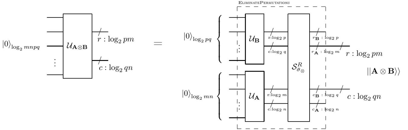
Figure 8: Graphical description of `qmsla.kronecker` (Input:  $\mathcal{U}_{\mathbf{A}}$  and  $\mathcal{U}_{\mathbf{B}}$ , Output:  $\mathcal{U}_{\mathbf{A} \otimes \mathbf{B}}$ ).
