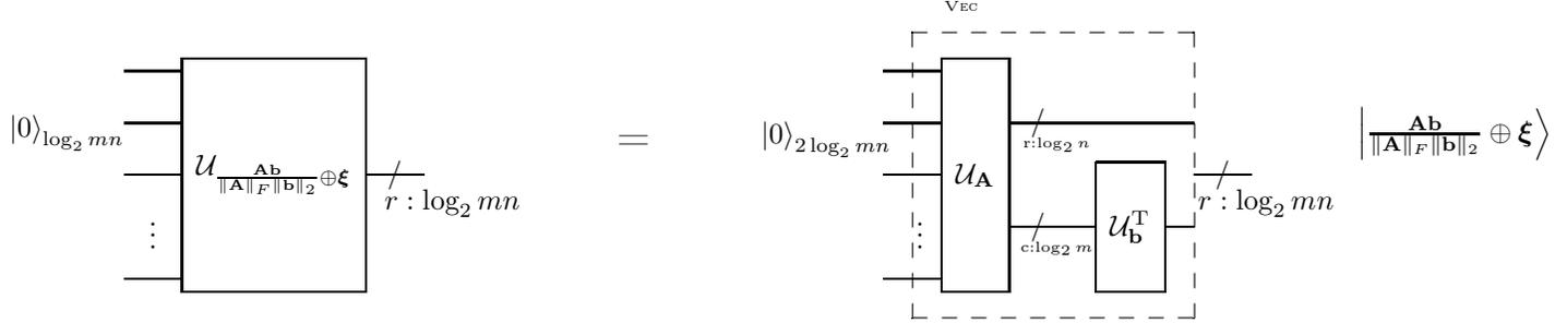
Figure 7: Graphical description of `qmsla.matrix_vec` (Input:  $\mathcal{U}_{\mathbf{A}}$  and  $\mathcal{U}_{\mathbf{b}}$ , Output:  $\mathcal{U}_{\frac{\mathbf{A}\mathbf{b}}{\|\mathbf{A}\|_F\|\mathbf{b}\|_2} \oplus \boldsymbol{\xi}}$ ).
