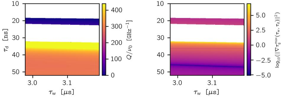
**Figure 3.** Normalized quality factor (left) and group delay gradient values of the DUT1 at  $N = 20$  as functions of the  $\tau_w$ —width—and  $\tau_d$ —location—parameters of a discrete prolate spheroidal sequence (DPSS) window, which is used to isolate the DUT response by time-domain gating. The lowest group delay gradient— $\|\nabla\tau_g^{\max}(\tau_w, \tau_d)\|^2$ —is used to select the actual  $Q$  value. White regions represent discarded negative and off-center  $Q$  values.
