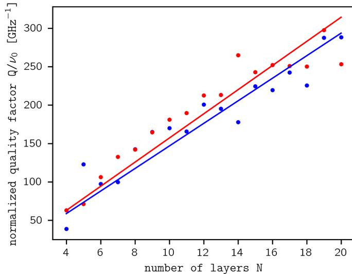
**Figure 4.** Measured quality factors of two fixed-plate dielectric haloscopes holding  $N$  layers with dimensions  $100 \times 100 \times 1$  mm constructed with 3 mol% yttria-stabilized zirconia with two different layer spacings, normalized to the resonant frequency,  $\nu_0$ . The measurements of DUT1 are shown in blue; those of DUT2 in red. The continuous lines represent the proportional fit reported in Table 1.
