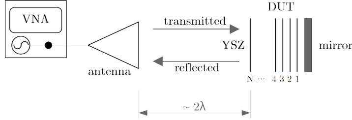
**Figure 2.** Schematic representation of the experimental setup for the measurement of the quality factor of the Fabry-Pérot resonators. A horn antenna placed at a distance of about  $2\lambda$ —beyond the lower limit of the radiative near field—excites the resonator with a signal generated by a VNA, which traverses the YSZ plates and bounces off the bottom mirror; a standing wave is created and picked up by the antenna, which is registered by the VNA as a reflectivity scattering parameter.
