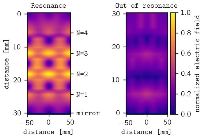
**Figure 5.** A finite element method simulation of the normalized electric field plotted on the transversal plane of a four-layer Fabry-Pérot interferometer at the  $\lambda/8$  resonant frequency (left) and out of resonance (right). The wavelength is  $\lambda \approx 4$  cm. The locations of the layers ( $N = 1, \dots, 4$ ) and the mirror are shown.
