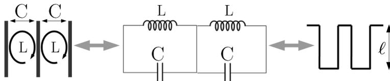
**Figure 7.** A series circuit for a Fabry-Pérot resonator and the performed transformations. Left: the multilayer resonator. Each layer is modeled as a capacitor (C) plus an inductor (L). Middle: LC equivalent circuit with lumped elements. Right: equivalent distributed elements.
