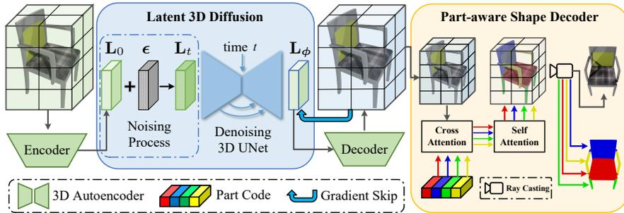
**Fig. 1:** The proposed method comprises two main modules: a latent 3D diffusion model and a part-aware shape decoder. The latent 3D diffusion model facilitates high-resolution generation of neural voxel fields, while the part-aware shape decoder enables the generation of parts-aware results for rendering. The two modules are trained in an end-to-end fashion.
