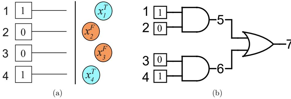
Figure 2: (a) The input bits of a threshold formula and their representation as species. (b) An indexed threshold formula with the input species shown in Figure 2a.
