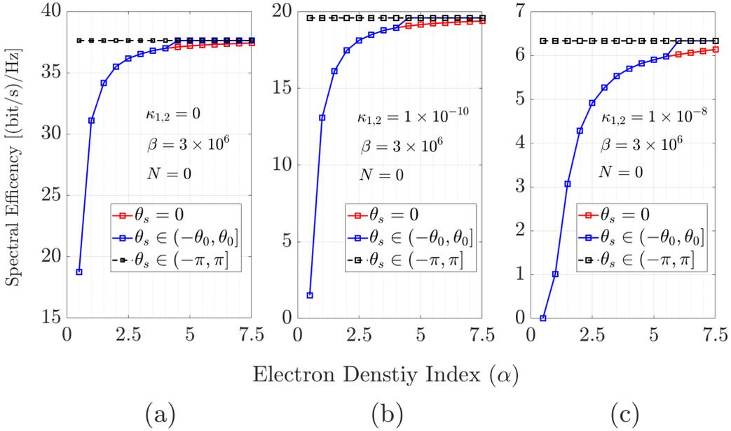
Figure 8. Expected spectral efficiency with ideal beamsteering of  $\theta_s$  without scan loss.
