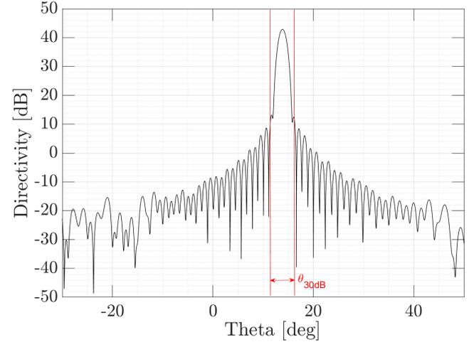
Figure 6. Directivity of the designed planar reflectarray with  $\theta_{ref}$  wave angle.
