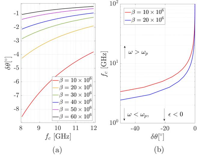
Figure 5. (a) The vulnerability to diffractions on the carrier within different solar plasma levels. (b) Robustness of the high-frequency band against X-band in solar plasma density.
