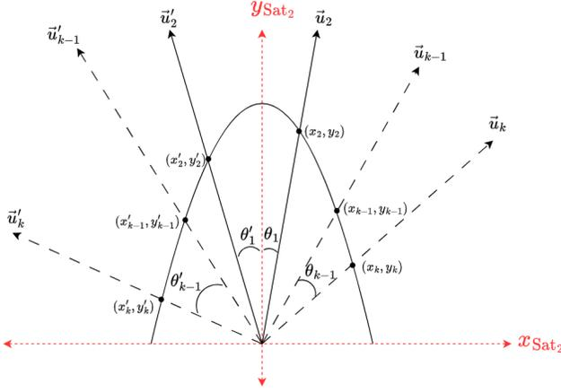
Figure 2. Finite spatial regions of asymmetric main beam radiation of Sat2 on local frame where each  $\vec{u}_i$  starts at the origin and  $y_{\text{Sat}_2}$  is the beam direction axis.
