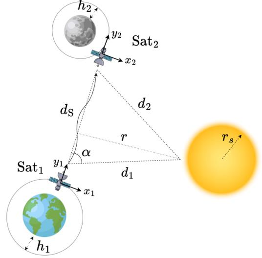
Figure 1. An IP-ISL of Sat<sub>1</sub> – Sat<sub>2</sub> on free space including the Sun, Earth and the Moon. Assuming orbital inclinations to be zero allows a simplified 2D model in the  $xy$ - plane. The diffracted trajectory along the Sat<sub>1</sub> – Sat<sub>2</sub> path due to  $\Delta\epsilon$ , leading to  $\delta\theta$  fluctuation on AoA.
