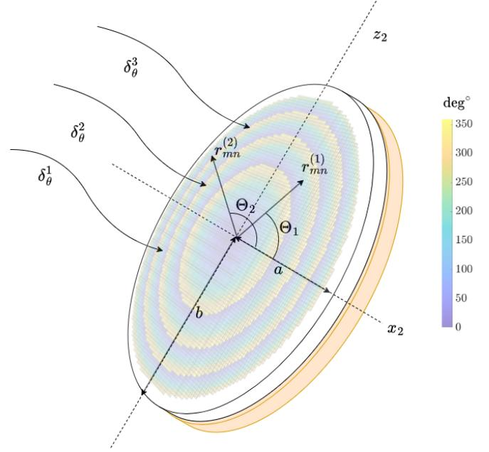
Figure 3. Angle of arrival fluctuations arise from the non-constant dielectric of the free space plasma within a time instance of the reflectarray aperture phase distribution.
