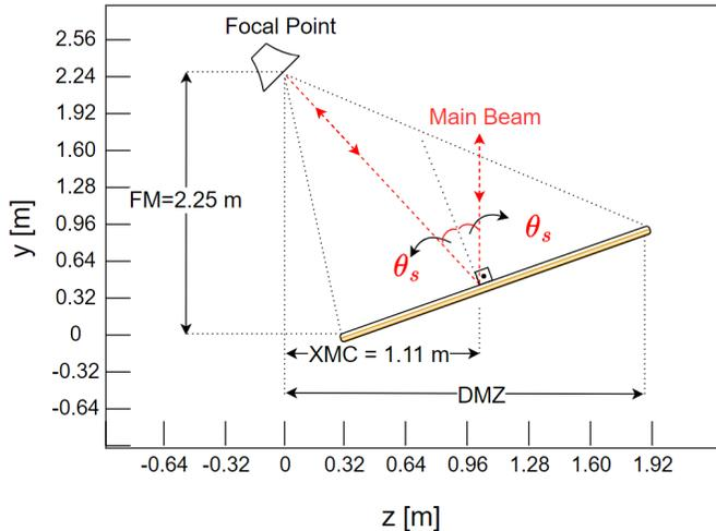
Figure 4. Planar reflectarray geometry design for both Sat<sub>1</sub> and Sat<sub>2</sub>.
