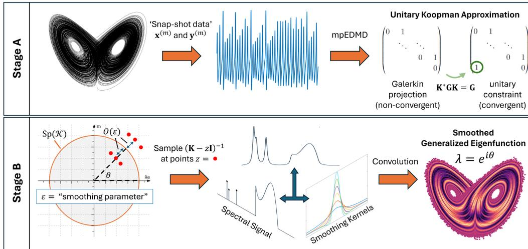
**Figure 1.** Schematic of Rigged DMD. Stage A consists of a data-driven unitary approximation of  $K$ . Stage B consists of sampling the resolvent of this approximation to form a smoothed generalized Koopman eigenfunction (and Koopman modes) in the form of a wave-packet approximation. These generalized eigenfunctions provide a decomposition, even in the presence of continuous spectra. The full algorithm is given in [Algorithm 3.1](#).
