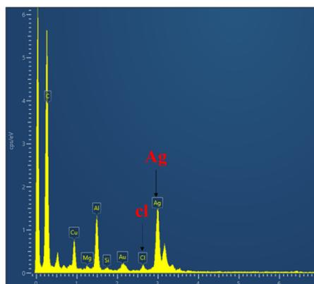
**Figure 3.** EDX analysis of synthesized Silver Shell™ solution.
