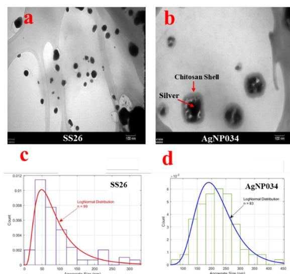
**Figure 2.** TEM images of a) SS26, b) AgMP034; Log Normal Distribution of c) SS26, d) AgMP034.
