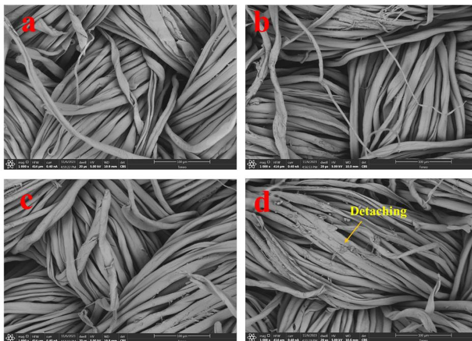
**Figure 5.** SEM images of AgMP034 with different washing cycles: a) no washing, b) 25 cycles, c) 50 cycles, d) 75 cycles.
