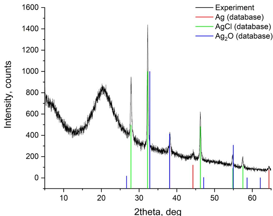
**Figure 1.** PXRD plot for the annealed Silver Shell™ solution.
