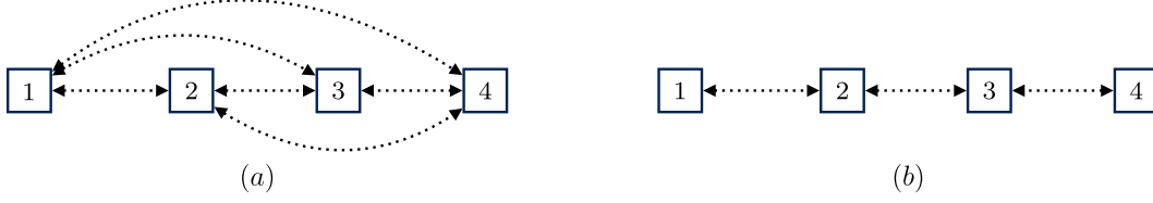
Figure 13. Communication links need to achieve (a) centralized and partially nested information exchange and (b) local information exchange for the serial energy hub system.
