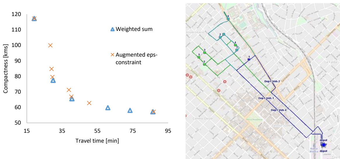
Figure 1. Pareto front of the proposed instance with 9 nodes (left) and non-dominated route of that front that provides a good trade-off between objectives (right).
