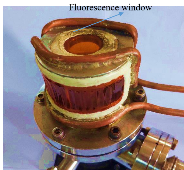
Fig. 3.7: Top Kapton window for the x-ray fluorescence measurements.
