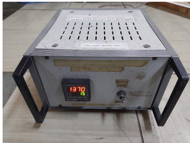
Fig. 3.3: Homemade PID controller for the precise temperature control of the heater.
