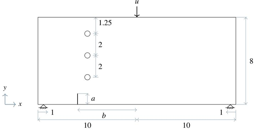
Figure 2: Parametrized geometry of the 3-point bending experiment. With Parameters  $a$  for the length and  $b$  for the position in  $x$ -direction of the initial crack. The values for the three cases are shown in Table 1. Adapted from [3].
