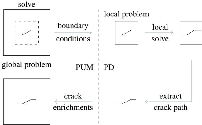
Figure 1: The combined PUM/PD simulator. Adapted from [4].
