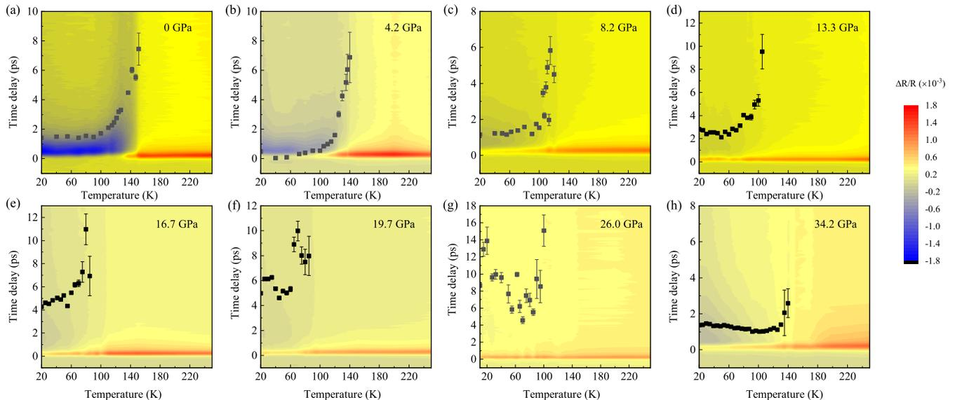
FIG. 2. Temperature dependent pump probe spectra taken at (a) 0 GPa, (b) 4.2 GPa, (c) 8.2 GPa, (d) 13.3 GPa, (e) 16.7 GPa, (f) 19.7 GPa, (g) 26 GPa and (h) 34.2 GPa. The scatters in each panel are the extracted  $\tau_s$ .
