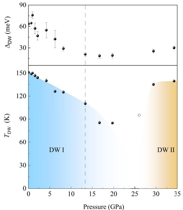
FIG. 4. Temperature-pressure phase diagram of the  $\text{La}_3\text{Ni}_2\text{O}_7$  based on the pump probe spectroscopy measurements. The upper panel shows the evolution of the extracted gap as a function of pressure.
