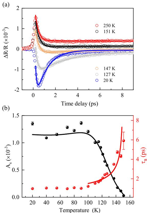
FIG. 1. (a)  $\Delta R / R$  signals at several selected temperatures and ambient pressure. The solid lines are the fitting curves. (b) Temperature dependent amplitude  $A_s$  and relaxation time  $\tau_s$ . The solid lines are fitting results according to RT model.
