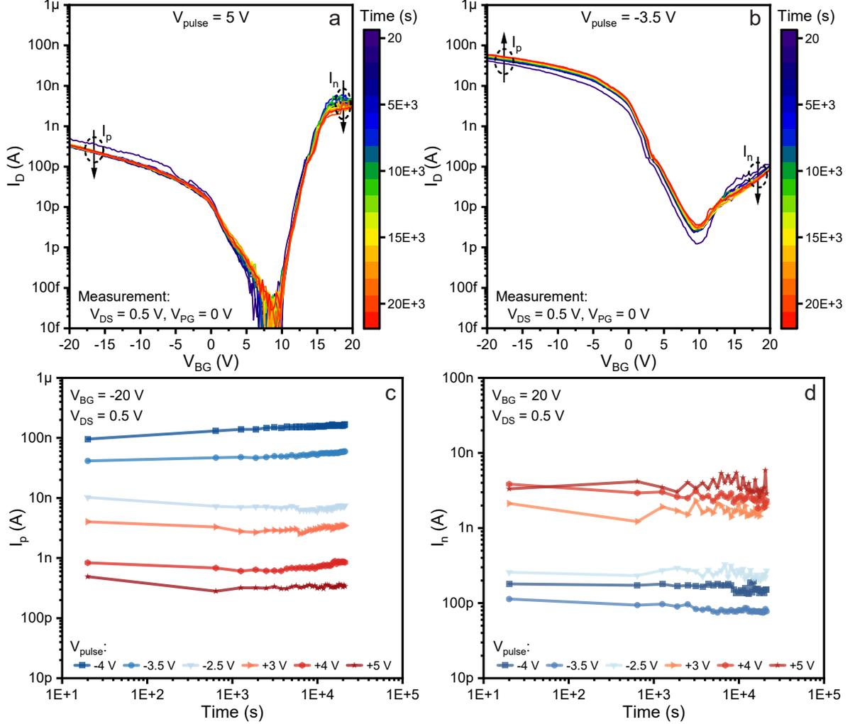
Figure 3: a) The device is polarized using a pulse height of +5 V. The panel reports several transfer curves measured every 15 min, up to 6 hours, showing little change. b) same as a, but after polarizing the device with a pulse height of -3.5 V. c) Time-dependency of the drain currents measured at p-side ( $V_{BG}=-20$  V) for different polarization pulse heights. d) Time-dependency of the drain currents measured at n-side ( $V_{BG}=+20$  V) for different polarization pulse heights.
