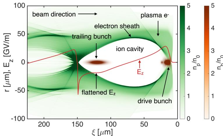
*Fig. 1. Schematic of two-bunch plasma wakefield acceleration. An intense beam (drive bunch) ionizes lithium vapor to create plasma (illustrated by the green colormap) and excites a wake, characterized by an ion cavity enclosed by a plasma electron sheath. The red line indicates the*
