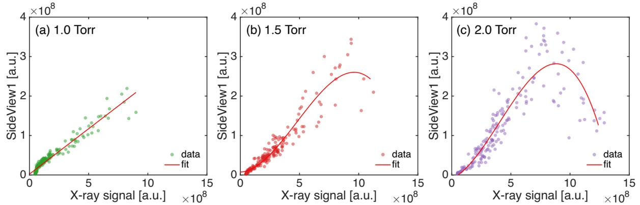
*Fig. 6. Correlation between plasma light and x-ray signal. The plasma light detected by the sideview1 camera is plotted as a function of the x-ray signal for three datasets acquired at different pressures. The red lines are polynomial fits [with order one (linear) for (a) and three (cubic) for (b) and (c)] to illustrate the trend of the data.*
