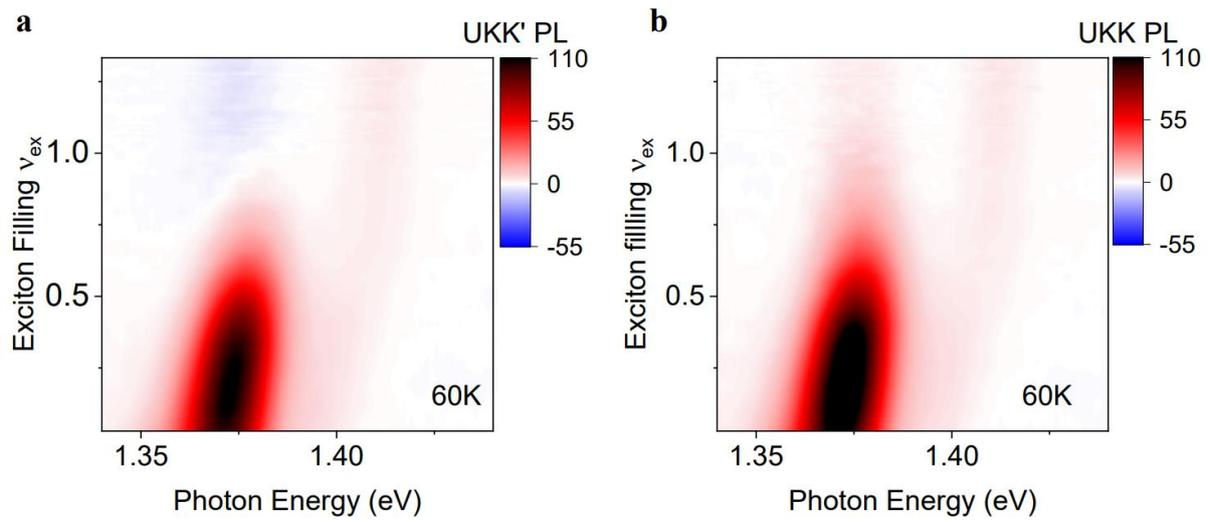
**Extended Data Fig. 5: Polarization-resolved probe-induced PL spectra of device D1 at 60 K.** The bosonic correlated insulator state and on-site AFM interaction are still robust at 60 K. UKK (UKK') refers to pump injecting unpolarized excitons, probe injecting  $K$  valley excitons and PL detecting  $K$  ( $K'$ ) valley excitons.
