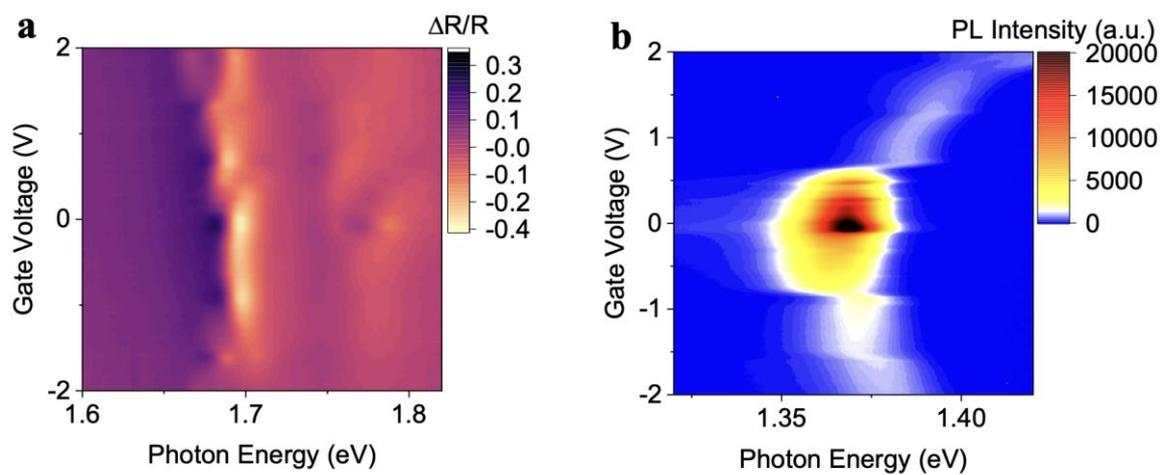
**Extended Data Fig. 3: Optical characterization of device D2.** Doping-dependent absorption (a) and PL (b) spectrum of the 0-degree aligned WSe<sub>2</sub>/WS<sub>2</sub> device D2 at zero pump intensity.
