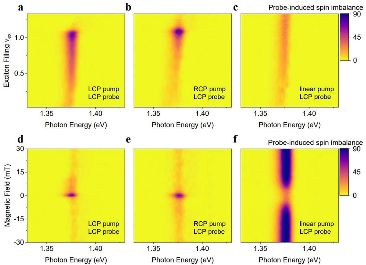
**Extended Data Fig. 4: Probe-induced spin imbalance in device D2.** **a-c**, LCP probe-induced spin imbalance as a function of background exciton fillings for LCP (**a**), RCP (**b**) and linear (**c**) pump respectively. **d-f**, Evolution of spin imbalance signal at  $\nu_{ex}=1.1$  under out-of-plane magnetic field  $B_z$  for LCP (**d**), RCP (**e**) and linear (**f**) pump, respectively.
