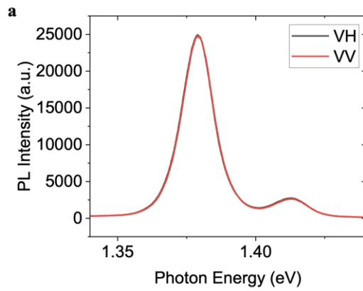
**Extended Data Fig. 8: Linear polarization-resolved PL at  $\nu_{\text{ex}} = 1.1$ .** No linear helicity is observed between vertical (VV) and horizontal (VH) PL detection, indicating that there is no global long-range FM- $xy$  order. The pump light is linearly polarized along the vertical direction.
