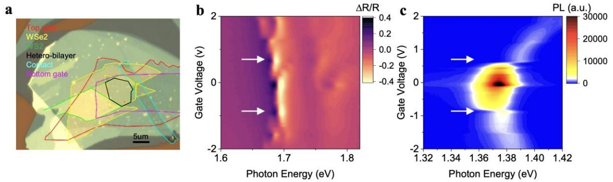
**Extended Data Fig. 1: Basic characterizations of devices.** **a**, optical image of a representative dual-gated 0-degree-aligned WSe<sub>2</sub>/WS<sub>2</sub> device D1. Yellow and green solid lines denote contours of the monolayer WSe<sub>2</sub> and WS<sub>2</sub> flakes, respectively. **b,c**, Electron doping-dependent absorption (**b**) and PL (**c**) spectrum of device D1 at zero pump intensity. White arrows indicate one filling of electrons and holes.
