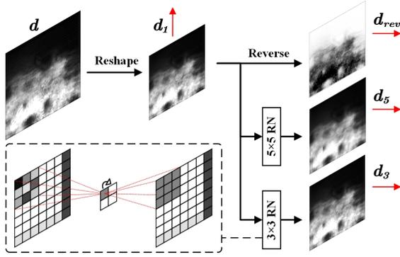
Fig. 3. R<sup>3</sup>N transformation of a depth map. The input is the depth map  $d$  and the outputs are the feature maps  $d_{rev}$ ,  $d_1$ ,  $d_3$ , and  $d_5$ . The process within the dashed line is a  $3 \times 3$  region normalization (RN).
