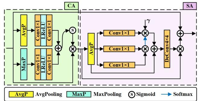
Fig. 4. Structure of the Dual-Attention Module (DAM)
