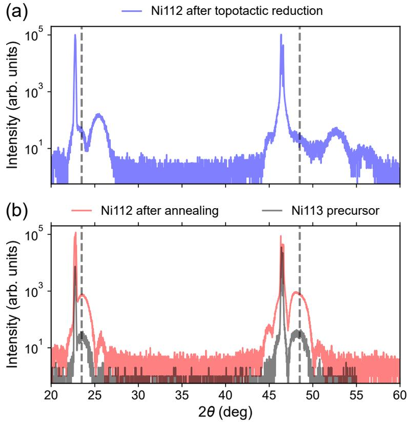
FIG. S2. Room temperature  $2\theta$  scans recorded on  $\text{PrNiO}_2$  (Ni112) and  $\text{PrNiO}_3$  thin films with crystalline STO capping layer. (a) Infinite layer phase Ni112 obtained after topotactic reduction of the perovskite precursor  $\text{PrNiO}_3$  (Ni113). (b) Comparison of the Ni112 thin film after annealing at high temperatures with the original Ni113 phase. The scans were performed using a SmartLab x-ray diffractometer with a  $\text{Cu K}\alpha$  source.
