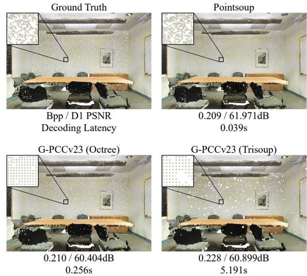
Figure 1: Quantitative compression results of proposed Pointsoup and G-PCCv23. Colors are rendered by nearest mapping. The “conferenceRoom\_1” in S3DIS Area 6 is used as an example, which has 1,067,709 points. Our method allows for the decoding of a million-scale point cloud geometry in 39 ms with only one **RTX 2080Ti GPU** while guaranteeing superior visual quality.
