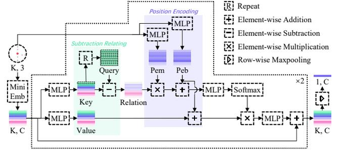
Figure 4: Attention-based aggregation of AWDS module. The self-attention block is presented in the dotted line.
