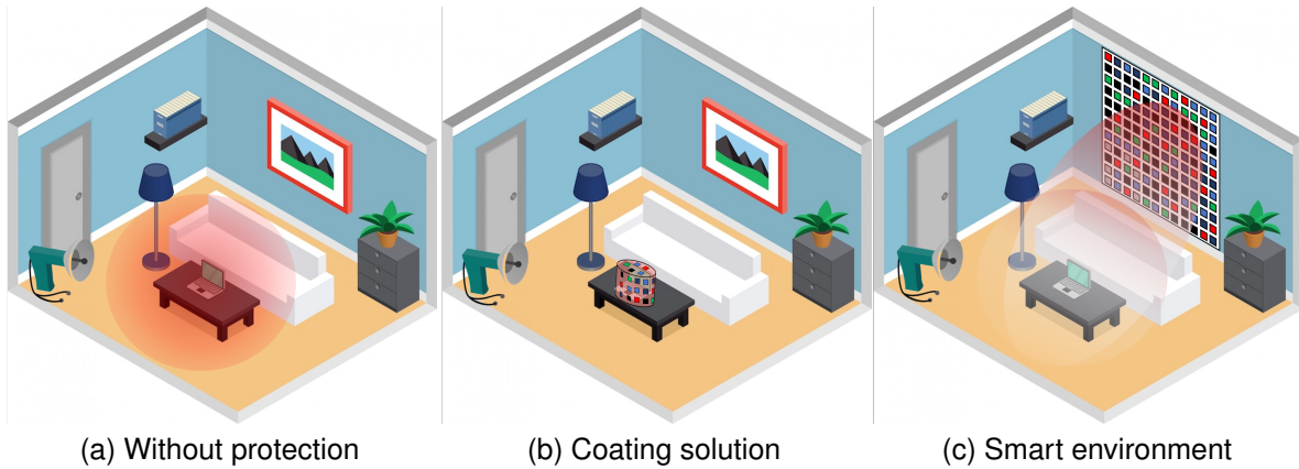
Fig. 4. Comparison of different object illusions in multi-reflective environment. In the cloaking case, the object is coated by conformal metasurfaces to engineer the backscattering but in the smart environment, the metasurface on the wall cancels out the scattering of the device.
