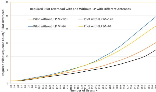
Fig. 4. Required pilot overhead with and without ILP
