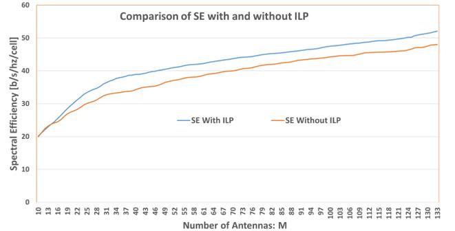
Fig. 3. Comparison of SE with and Without ILP
