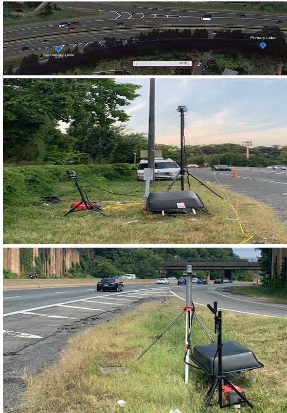
Fig. 3: The data collection setup (top) included two lidar sensors placed on the side of the road: a 128-beam primary lidar placed near the merging area (middle) and a 32-beam secondary lidar placed further down the road (bottom). Each lidar sensor was mounted on a base station mast, which included a camera platform, power supply, cellular WiFi router, data acquisition server, and monitor.
