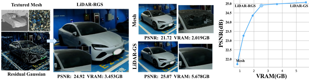
Figure 4: Our LiDAR-RGS system comprises a base mesh, a series of residual Gaussians, and a blending weight map. These components enable our system to maintain a photorealistic appearance comparable to LiDAR-GS while significantly reducing runtime memory. This approach strikes an optimal balance between memory consumption and visual fidelity.
