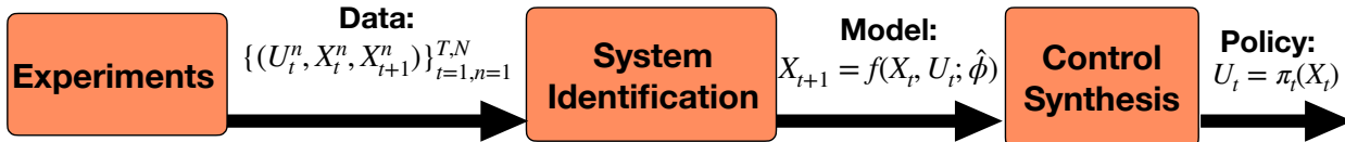
Figure 1: Identification to control pipeline.
