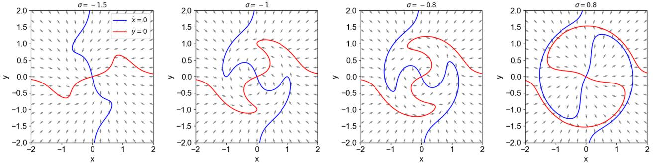
Fig. 1. Nullclines and vector fields of the system (1) in different parameter regimes. In all cases,  $a = 1, b = 1$ , and  $\omega = 0.4$ .
