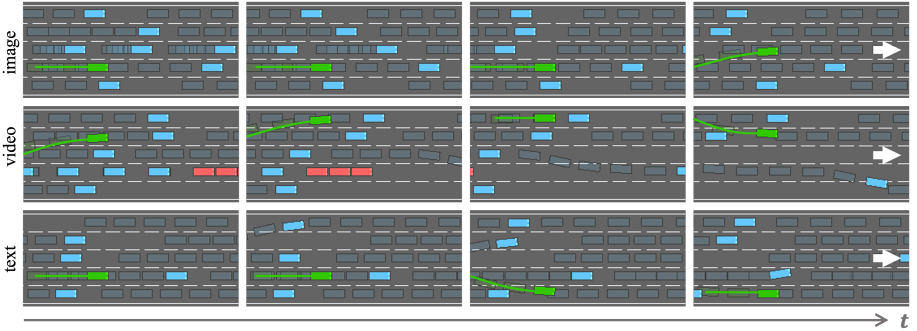
Fig. 5: Illustrations of how the driving policy learned by our LORD with image, video and text based observation performs in the lane-5-density-3 setting of Highway-env. The ego vehicle is colored in green with a line depicting its past trajectory. The ego vehicle behaves properly in the congested traffic scenarios.
