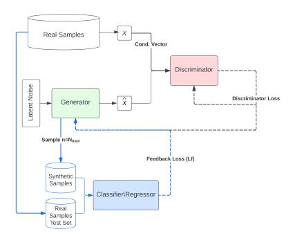
Figure 1: Downstream Feedback Generative Adversarial Network Schematic Flow
