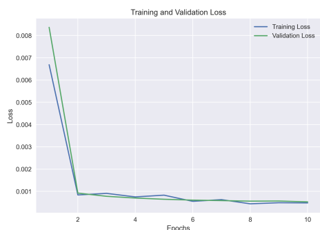
Figure 4: Loss graphs (MSE) for training and validation varied with number of epochs for task 2 using the most optimal hyperparameter found. The loss converges very quickly after the first two epochs.
