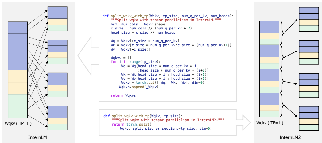
Figure 2: Different weight matrix layouts cause different complexity when changing the tensor parallelism (TP) size.
