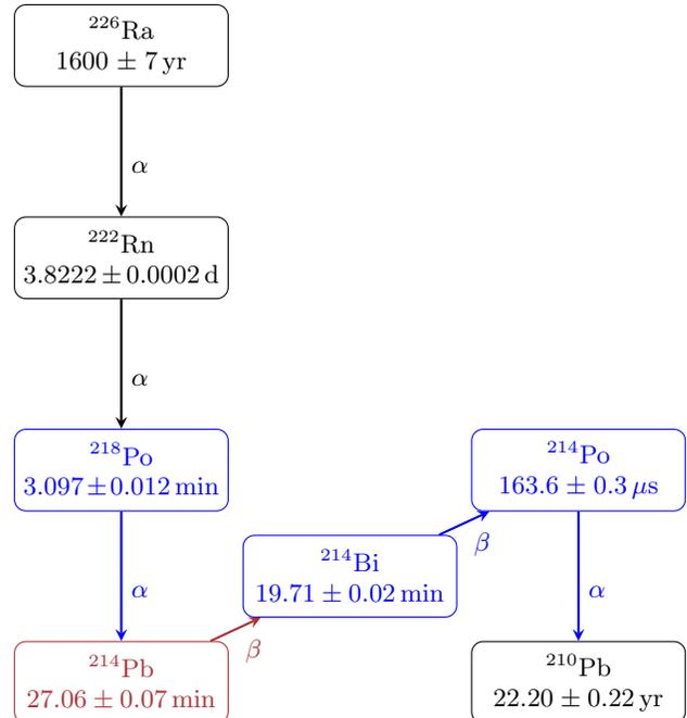
FIG. 1. Decay chain of  $^{222}\text{Rn}$ , part of the uranium series. Only branches with branching fraction above 99.5% are shown. Data retrieved using the NNDC ENSDF, with the following Nuclear Data Sheets citations: [14, 29–32]. The isotope that decays to produce the background events being tagged in this work,  $^{214}\text{Pb}$ , is coloured red, whereas the isotopes with decays that are used for the tagging of  $^{214}\text{Pb}$  are coloured blue.
