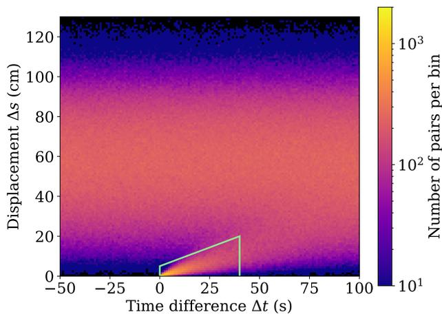
FIG. 2. 2D histogram of the time difference ( $\Delta t$ ) and displacement ( $\Delta s$ ) of all permutations of  $^{222}\text{Rn}$  and  $^{218}\text{Po}$  pairs. The excess of pairs where  $\Delta s < 20$  cm and  $0 \text{ s} < \Delta t < 40 \text{ s}$ , is from correctly-paired events, and is highlighted with the light green box. At negative times, the pairs are unphysical and can be used to profile the distribution of incorrect pairs.
