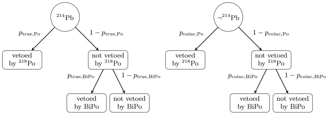
FIG. 10. Tree diagrams describing the probabilities involved in whether  $^{214}\text{Pb}$  events (left) and other events (right) are vetoed, given both  $^{218}\text{Po}$  and BiPo channels. This tree diagram describes the derivation of Equation (6). An event is vetoed if the veto is triggered by either the  $^{218}\text{Po}$  or BiPo channels.
