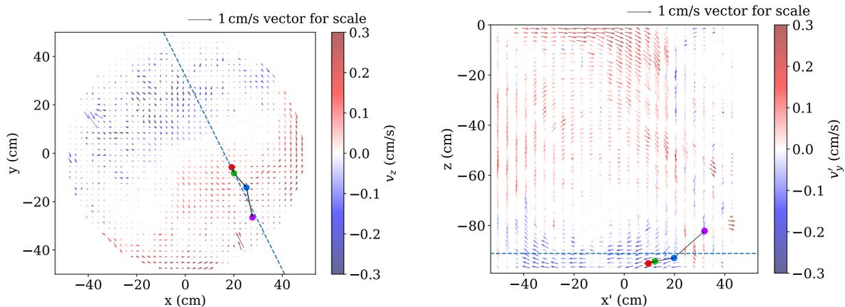
FIG. 15. The positions of a  $^{222}\text{Rn}$  event (red), a  $^{218}\text{Po}$  event (green), a  $^{214}\text{Pb}$  event (blue), and a BiPo event (purple) are shown here, overlaid on top of the velocity field in the detector. The top view is shown on the left, and a side view is shown on the right. The blue dotted line on the top and side views are used to show the slices taken to create the side and top views, respectively.
