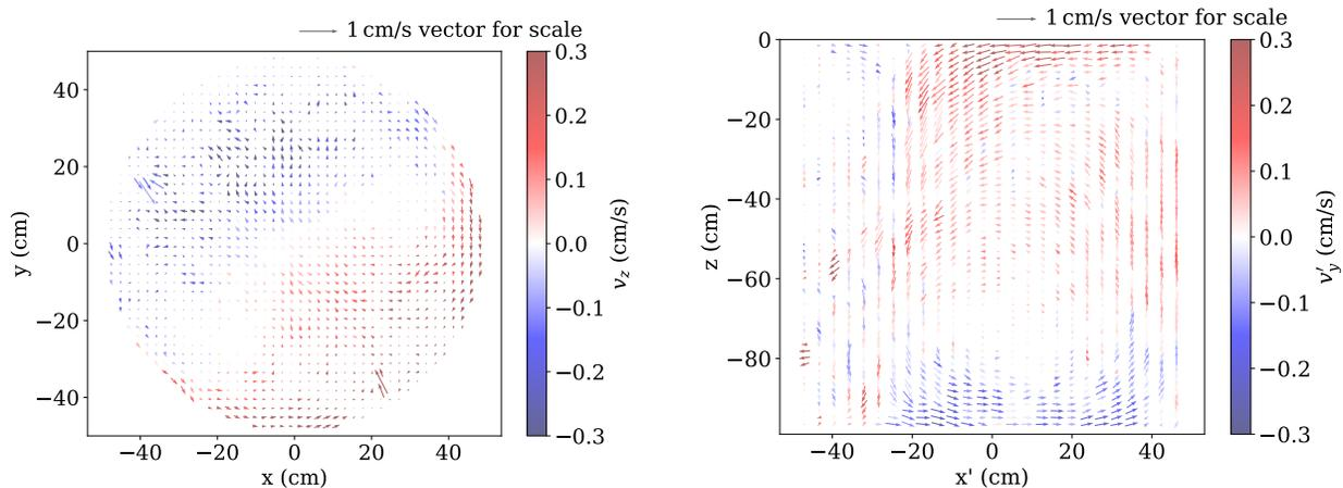
FIG. 4. Slice of the velocity field after it was filtered and put discretized onto a grid, shown from the top view (left) and the side view (right). In the left plot, the  $x'$  coordinate is defined as in Figure 3; in the right plot, a slice at  $z = -50$  cm is taken. For clarity, only every 6th vector is displayed. A 1 cm/s velocity vector is shown in the top right for scale.
