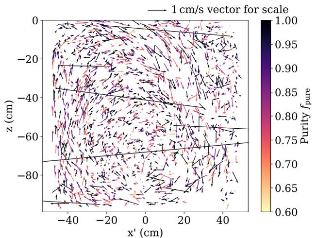
FIG. 3. Slice of velocity field with 107804 vectors showing the convection cell. The  $x'$  coordinate is perpendicular to the angular momentum vector. A 1 cm/s velocity vector is shown in the top right for scale. The purity of a vector,  $f_{\text{pure}}$ , is indicated by the colour.
