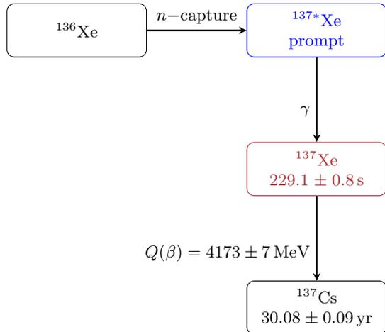
FIG. 18. Neutron capture of  $^{136}\text{Xe}$  and subsequent decay of  $^{137}\text{Xe}$ . Data regarding the decay of  $^{137}\text{Xe}$  and  $^{137}\text{Cs}$  retrieved using the NNDC ENSDF, with original data from Nuclear Data Sheets [58]. The isotope the decays to produce the relevant background,  $^{137}\text{Xe}$ , is coloured red, whereas the excited state which produces the gamma events that are used for the tagging of the  $^{137}\text{Xe}$  background are coloured blue.
