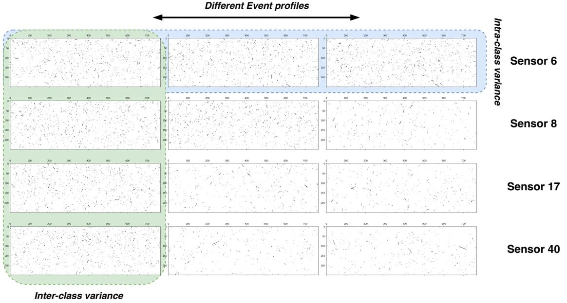
Figure 5.4: PXD background signatures across events for different sensors. The horizontal cases demonstrate various profiles (different clustering, occupancy, etc.) across different events. The vertical cases exhibit similar profiles across sensors.
