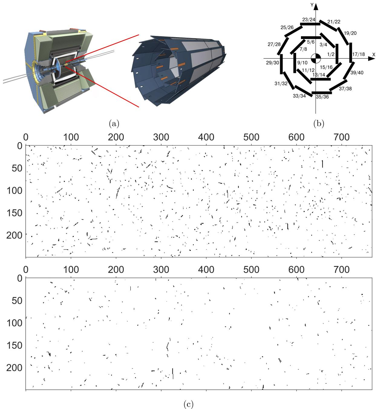
Figure 2.6: **Pixel detector layout** The pixel detector (PXD) is the inner-most sub-detector of the Belle II experiment (a) and is configured in a two-layered overlapping sensor structure (b). Geant4 Simulated PXD Background image examples (c) for sensors 7 (top) and 25 (down).
