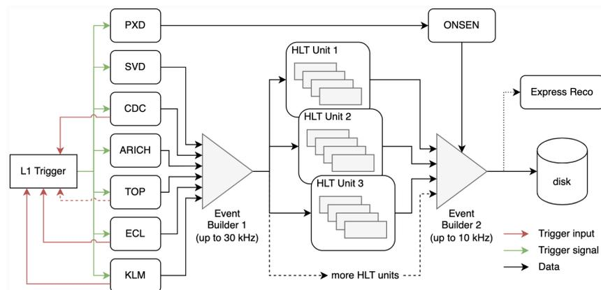
Figure 2.3: A schematic and simplified diagram of the Belle II data flow, taken from [15]
