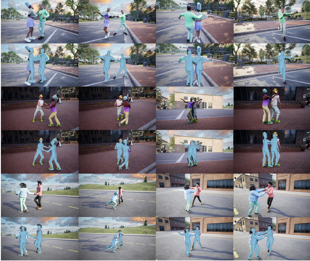
Figure 7: Visualization of camera space results on WHAC-A-Mole dataset. Each sample comprises two rows: the first row displays the original input frames from the sequence, while the second row overlays the SMPL-X results. This visualization showcases WHAC’s performance on challenging scenes, including sequences with severe occlusions, intricate human interactions, and dynamic dancing poses.
