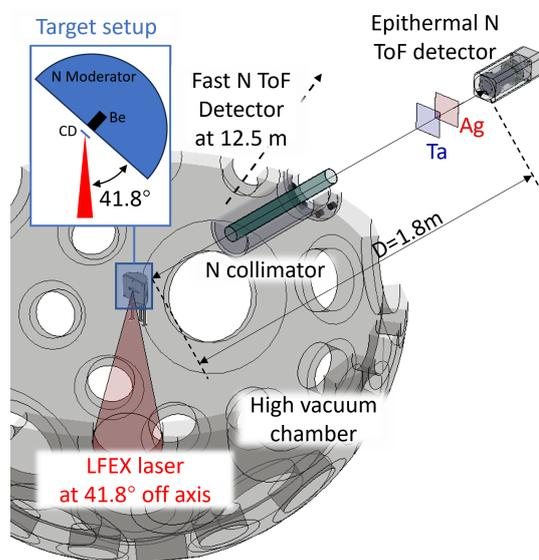
**Fig. 5** The structure diagram of neutron collimator used in LDNS experiments.
