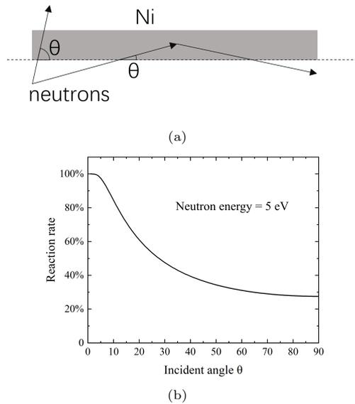
**Fig. 2** (a) The schematic diagram of nickle collimator. (b) The reaction rate of 5eV neutrons elastic scattering changes with incident angles.
