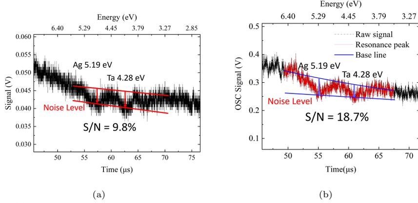
**Fig. 6** (a) The experimental result of NRS using LDNS without any shield and collimator. The resonance samples are Ag and Ta. (b) The experimental result of NRS using LDNS with the nickel collimator design above. The resonance samples are Ag and Ta.
