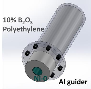
Fig. 4 The structure diagram of neutron collimator used in LDNS experiments.
