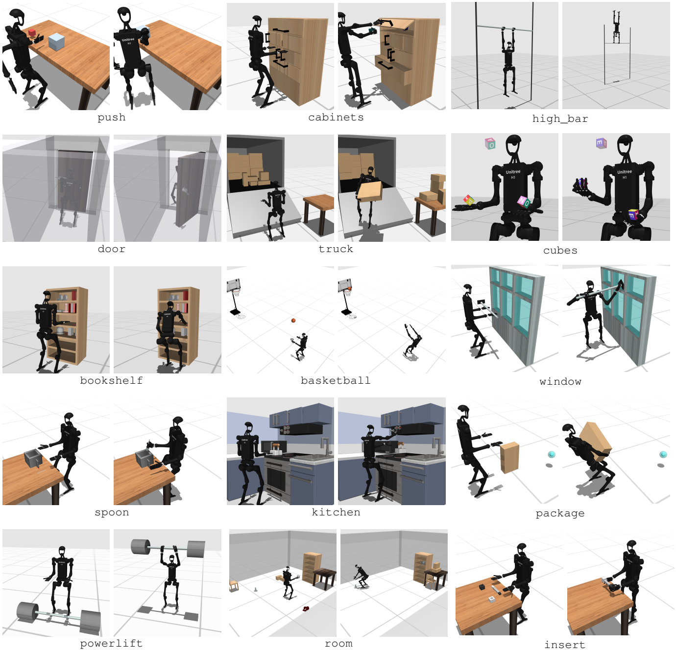
Fig. 3: HumanoidBench manipulation task suite. We devise 15 benchmarking whole-body manipulation tasks that cover a wide variety of interactions and difficulties. This figure illustrates an initial state for each task (left) and examples of the robot performing such tasks (right).
