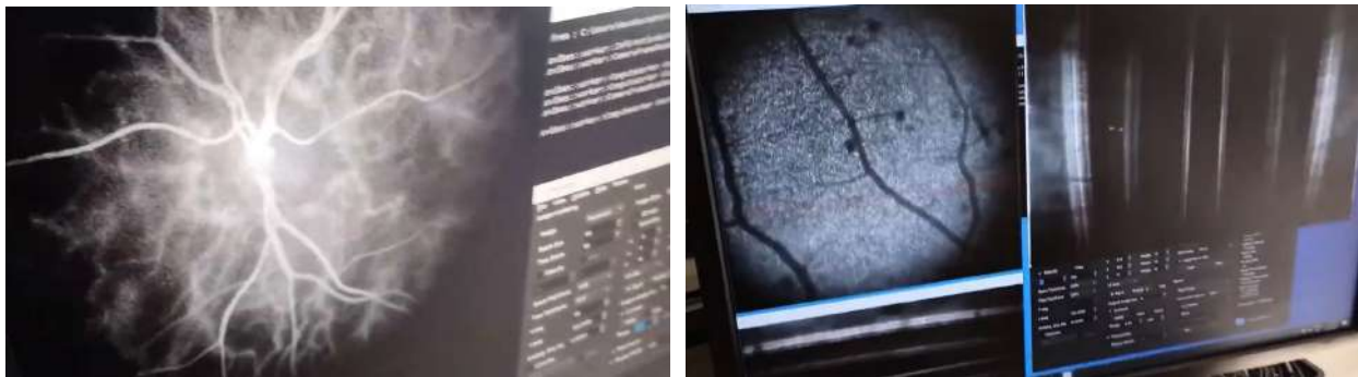
Fig. 24 : Real-time Doppler holography ( movie ) and holographic OCT ( movie ) at 20,000 frames per second (10 GB/s) with the software holovibes . OCT interferogram data is provided courtesy of Egidijus Auksorius and Maciej Wojtkowski.
