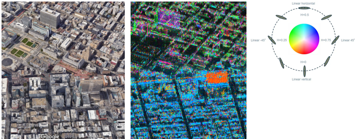
Figure 1: Left: Optical View of the neighborhood selected over San Francisco- Right: polarimetric representation of radar image selected. Hue represents the polarimetric orientation angle, Saturation is the temporal degree of polarization, and amplitude is the time-filtered amplitude.
