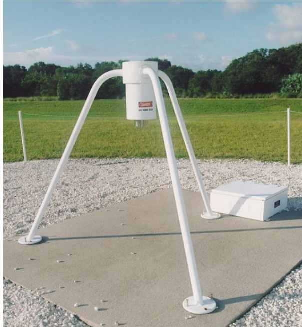
FIG. 2. One of the surface field mill machines located at the CCAFS/KSC. Photo courtesy of NASA (2006).
