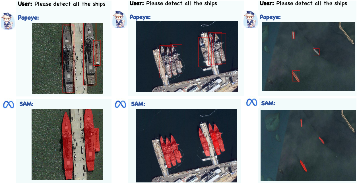
Fig. 3. Examples of language-referred pixel-level segmentation by integrating Popeye and Segment Anything Model (SAM).
