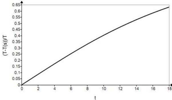
Fig.1. Dependence of the ratio of changes in the average lifetime  $\Delta T = T - T(s)$ , to  $T$ , where  $T$  is the average lifetime of the RV without taking into account radiation effects,  $T(s)$  – taking into account, on the reactor operating time  $t$  (in years),  $T_f = 40$  years,  $E_n = 1$  MeV,  $\sigma_n = 1 \cdot 10^{-26}$  cm<sup>2</sup>,  $T_e = 589$  K, fluence  $\Phi(t) = 0.98889t \cdot 10^{18}$  n cm<sup>-2</sup>, in the interval  $t = 0-18$  years.
